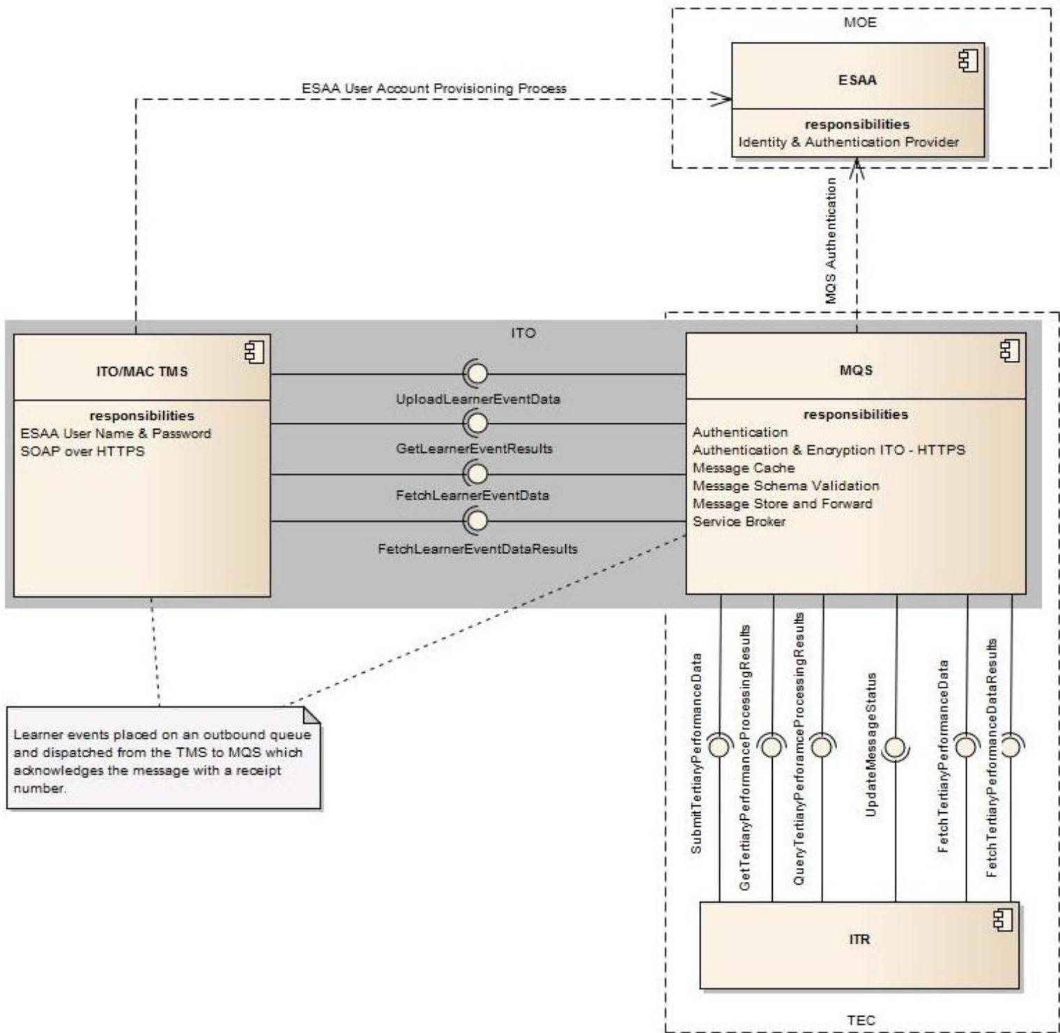
Learner events placed on an outbound queue and dispatched from the TMS to MQS which acknowledges the message with a receipt number.
